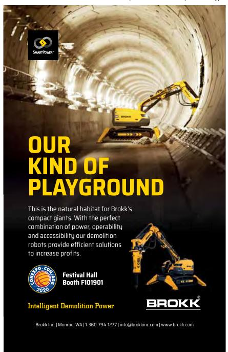
with the new Brokk BHB 305 breaker, the unit's hitting power is increased by 40%. The new class of machine delivers 450 foot-pounds (610 joules) with each blow of the 650-pound (295-kilogram) hydraulic breaker. Additionally, the Brokk 200 offers 15% longer vertical and horizontal reach in a compact footprint similar to the Brokk 170. The extra chassis length and machine weight ensures proper balance, even when wielding heavy attachments.
